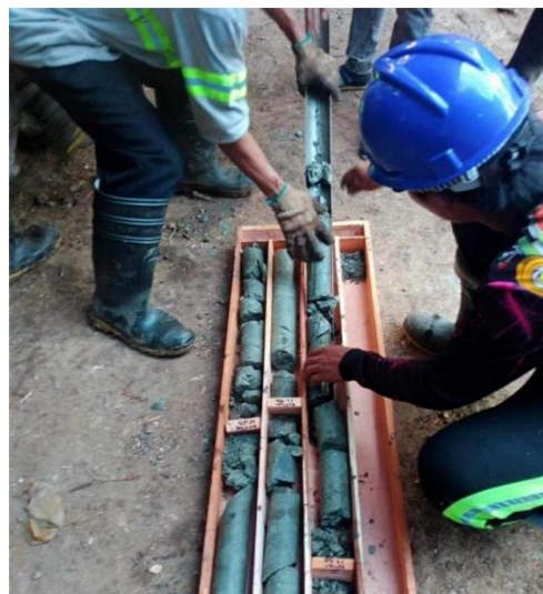
Drill core logging activities at Pan de Azucar February 2024
