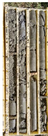
PDDH 24-04 (99.8m – 103.10m) massive pyrite
