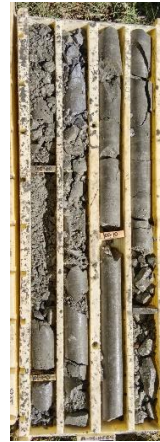
PDDH 24-04 (99.8m – 103.10m) massive pyrite
