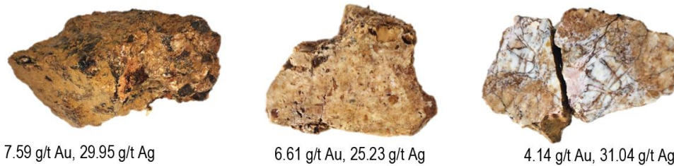
Figure 2. Quartz vein samples collected along the identified Daguman vein, found adjacent to the identified low magnetic anomaly zones. Quartz textures generally show chalcedonic to saccharoidal textures with minimal sulfides present
